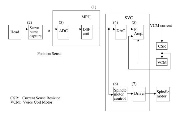
Figure 4.4 Block diagram of servo control circuit
